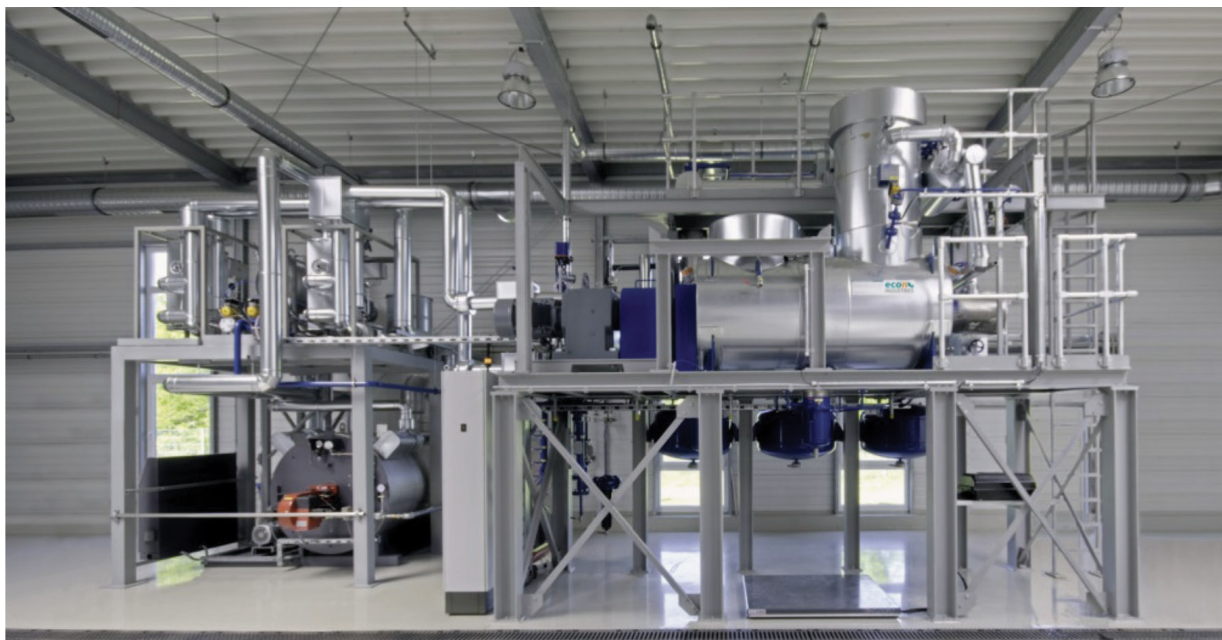
Figure 5-4: Mercury Recovery from Industrial Waste by Vacuum Thermal Processing (Source: Econ Industries)
