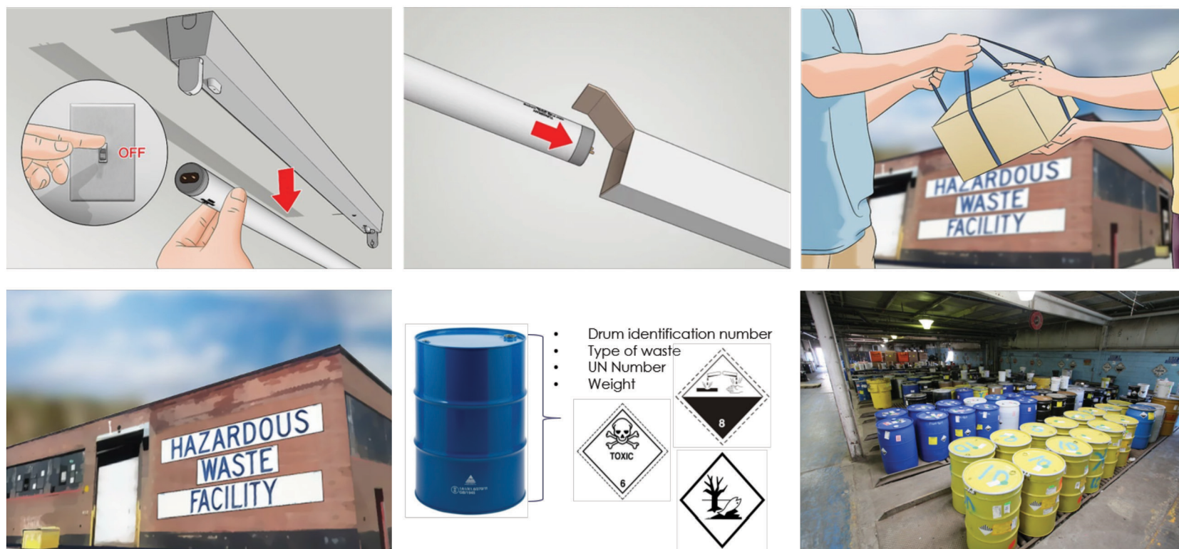
Figure 3-8: Example of a Waste MAPs being sent in original product packaging to a hazardous waste facility where it is labelled properly and kept for interim storage pending further operations for environmentally sound disposal (Source: BFS 2021)
